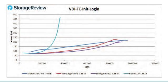
In VDI Full Clone Monday Login, the Solidigm P5520 started with a slightly elevated response time. However, as the workload increased, it offered a higher performance profile than others in the group. Here the P5520 measured 634k IOPS at 156 microseconds, with the 7400 Pro behind it with 606k IOPS at 166 microseconds.
