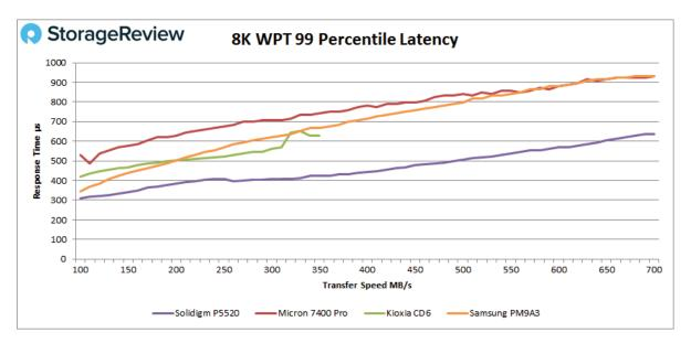
At the 99.9th percentile, we saw a more significant separation between the enterprise SSDs in this group. The P5520 started substantially lower than others in the group and maintained that lead across the test segment. If we look at the 350MB/s point, we measured 578 microseconds from the P5520, 922 from the CD6, 1,074 from the PM9A3, and 1,254 from the 7400 Pro.
