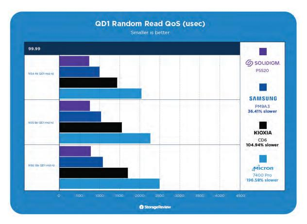
Moving to the six-9s or 99.9999 latency measurement, the P5520 continued its impressive lead over the group, measuring 1,123 microseconds. The Samsung PM9A3 remained in second place, measuring 1,494, the Kioxia CD6 jumped to 2,748, and the Micron 7400 Pro measured a staggering 3,796.
