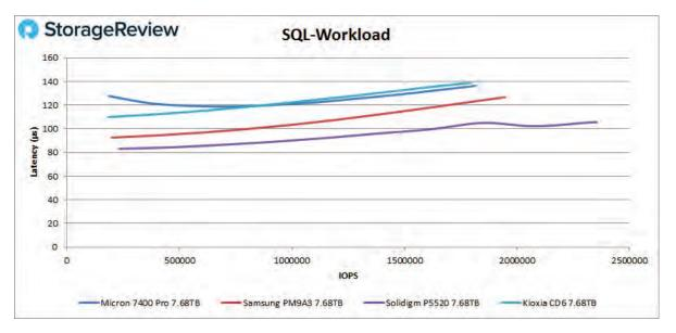
With an increased write percentage in our SQL 90-10 workload, the P5520 again offered a strong lead in front of the competing SSDs. Here we measured a peak of 2.23M IOPS at 111 microseconds, with the PM9A3 coming in behind it with 1.89M IOPS at 129 microseconds.
