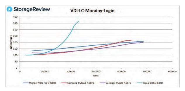
Finally, in our VDI Linked Clone Monday Login workload, we saw the Solidigm P5520 come through with a narrow lead on latency compared to the Micron 7400 Pro. Here the P5520 measured 485k IOPs at 198 microseconds, compared to 487k IOPS at 205 microseconds from the 7400 Pro.
