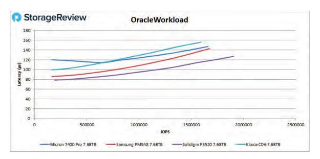
In our Oracle 90-10 workload, the P5520 topped out at 1.7M IOPS at 99 microseconds, with the PM9A3 as the next closest SSD, measuring 1.54M IOPS at 110 microseconds.
