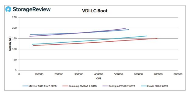
In the VDI Linked Clone Initial Login profile, the Solidigm P5520 came in just behind the PM9A3. The P5520 measured 312k IOPS at 148 microseconds, whereas the PM9A3 measured 325k IOPS at 140 microseconds.
